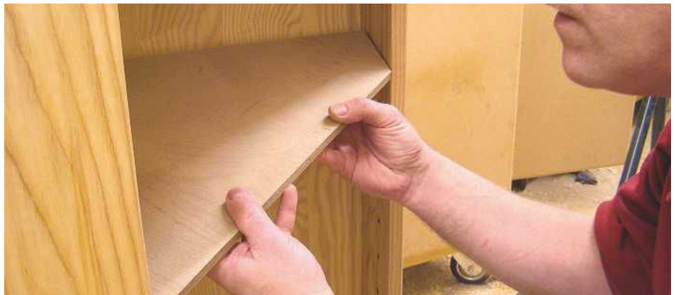
▲ Pic.18 Use an offcut of thin plywood to make an accurate template for the shelves, and cut them to size
